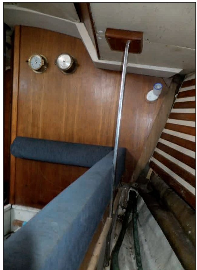
Figure 2: The starboard tie bar intact and in-situ
