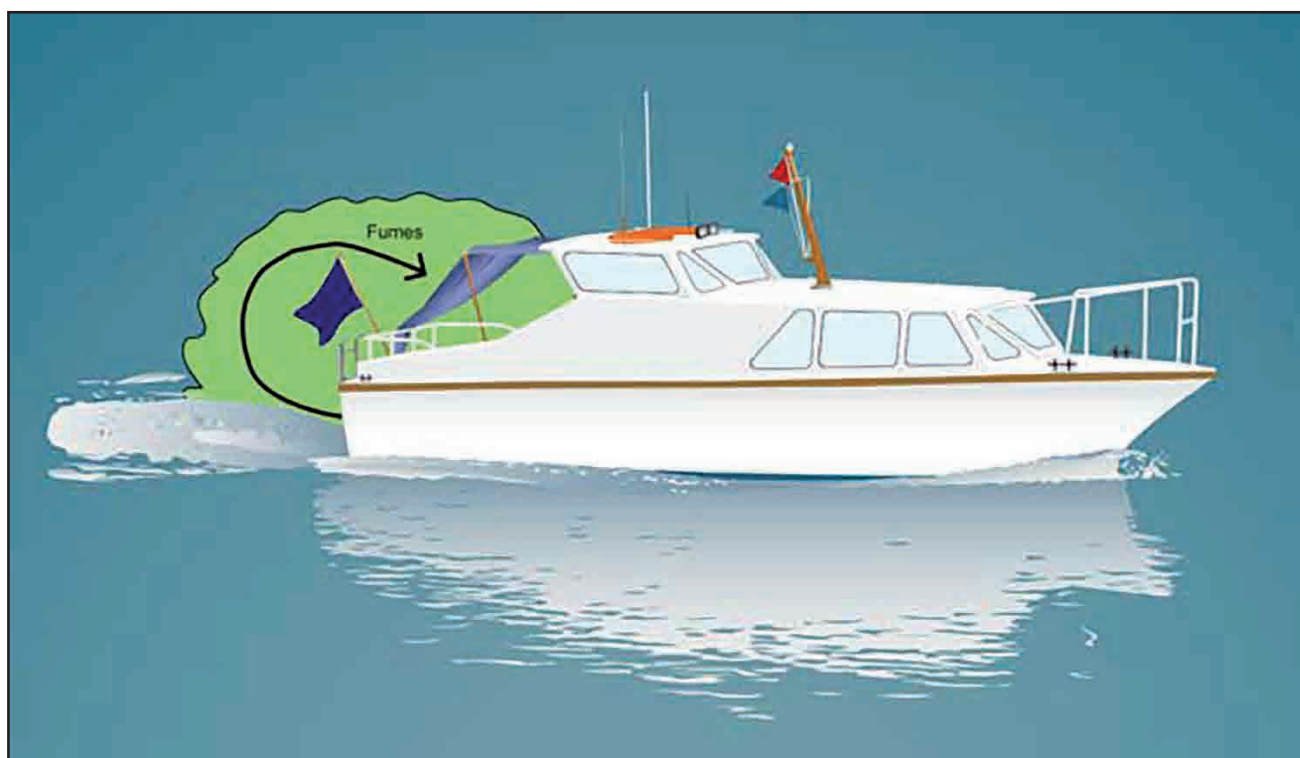
Figure 2: Diagram showing 'station wagon effect'
