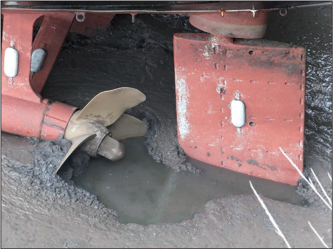
Figure 2: Damaged propeller and rudder
